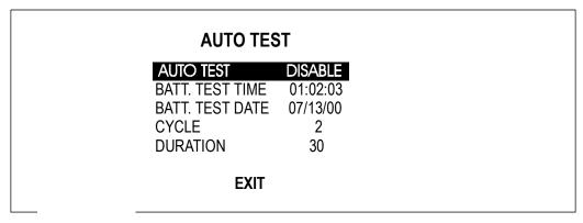
To enable the Auto Battery Self Test, Select "Auto Test Enable" from the Battery Test screen. Next, set the Date and Time at which the first test will be performed. Set the Test Cycle period in weeks. (The range is 2-9 weeks and the default is 2 weeks.) Finally, set the Test Duration time in seconds according to the table above. The range is 30-900 seconds and the default is 60 seconds. Use the UP DOWN navigation buttons to change the cursor position when setting battery parameters.
